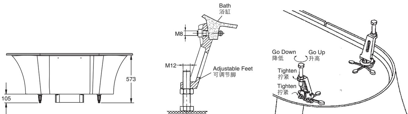
2. After the supports are adjusted, return the cast iron bathtub to its normal position with the bottom facing down as illustrated in the following figure. Shake the cast iron bathtub to verify whether the four supports are even. If the bathtub is shakable, it means that the floor is not sufficiently even. You can use a wrench to adjust 1 screw with the highest deviation so that the four supports are placed on the floor. Install and tighten the bathtub water drain and pull out the drainage pipe.
