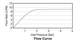
Note: 1. Flow rates are approximate. (1 gallon = 3.785 liters, 1 bar = 14.5 psi) 2. Flow curves above show the flow rate with the flow regulator installed.
