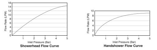
Note: 1. Flow rates are approximate. (1 gallon = 3.785 liters, 1 bar = 14.5 psi) 2. Flow rates shown with supplied flow regulators installed.
