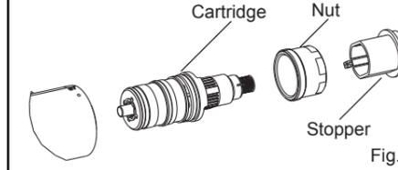
After cleaning, install the "stop assembly" back on the cartridge, adjusting the stop pin into the notch.
