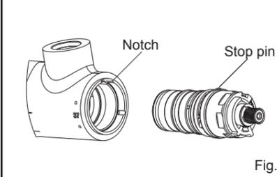
**NOTE:** Do not turn the cartridge when reinstall it. If you turned it without carefully, you should adjust it and be sure that the round mark is correctly in line with the groove, or readjust as per the steps of verification and setting.
