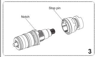
3. After cleaning, install the "stop assembly" back on the cartridge, adjust the stop pin into the notch.
