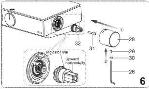
6. Install the adapter spline(without turning the spindle). Ensure the indicator line on the adapter spline align with the indicator line on the stopper. Tighten the screw(31) with a screwdriver. Install the temperature handle(28). Ensure the number 37 on temperature handle is upward vertically(After assembly, it could not be turned counterclockwise if not pushing the button). Tighten the screw (29) with 2.5mm hex wrench(26). Insert the plug(30).
