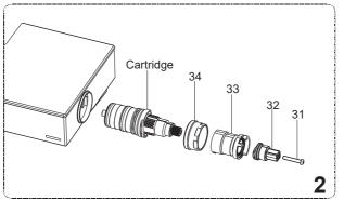
2. Remove the screw(31) and adapter spline(32), and then unscrew the nut(34) and stopper(33). Remove the cartridge cautiously. Clean the thermostatic cartridge by soaking it in warm vinegar.
