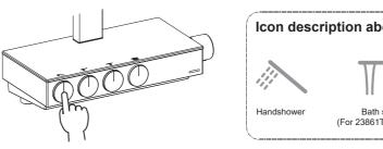
The temperature is set by slowly turning the temperature hand that limits temperature to 37°C. To get a higher temperature, p temperature handle counter-clockwise.
