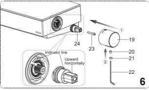
6. Install the adapter spline(without turning the spindle). Ensure the indicator line on the adapter spline align with the indicator line on the stopper. Tighten the screw(23) with a screwdriver. Install the temperature handle(19). Ensure the number 37 on temperature handle is upward vertically(After assembly, it could not be turned counterclockwise if not pushing the button). Tighten the screw (20) with 2.5mm hex wrench(22). Insert the plug(21).
