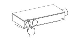
The temperature is set by slowly turning the temperature handle(right-hand handle). For safety reasons, there is a stop that limits temperature to 37°C. To get a higher temperature, push the button(on right-handle) and continue turning the temperature handle counter-clockwise.
