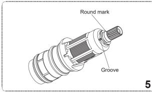
5. **NOTE:** Do not turn the cartridge when reinstalling it. If you turned it without carefully, you should adjust it and be sure that the round mark is correctly in line with the groove, or readjust as per the steps of verification and setting.
