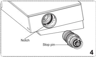
4. Install the assembly cartridge and stop in the body, adjust the stop pin into the notch.
