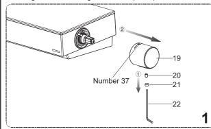
1. Before your action, make sure the number 37 on the temperature handle is upward vertically(It could not be turned counter-clockwise if not pushing the button). Remove the temperature handle(19).
