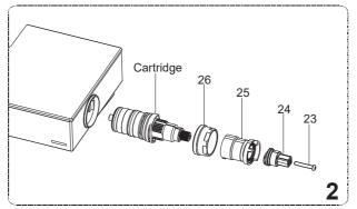
2. Remove the screw(23) and adapter spline(24), and then unscrew the nut(26) and stopper(25). Remove the cartridge cautiously. Clean the thermostatic cartridge by soaking it in warm vinegar.
