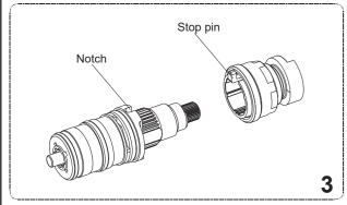
3. After cleaning, install the "stop assembly" back on the cartridge, adjust the stop pin into the notch.
