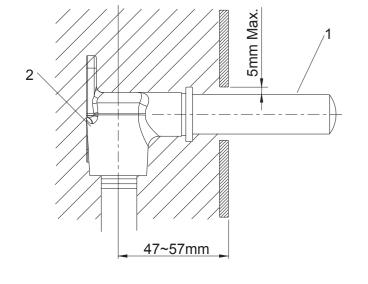
The distance between finished wall and supplies should be 47~57mm. Ensure that the gaps between guards and finished wall are less than 5mm.
