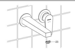
Ensure that all coupling nuts are tight. Ensure that the lever handle is in the off position.
