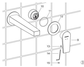
Be sure the O-ring(11) is in the groove of the escutcheon(12). Supply enough plumbers putty or other sealant to the rear of the escutcheon. Slide the escutcheon with o-ring onto the valve base(10) until it is against the wall.
