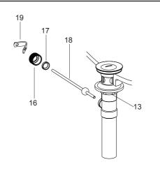
**NOTE:** Do not reposition the drain if plumbers putty applied after the locknut is tightened, or you may break the putty seal. Wipe away excess plumbers putty.
